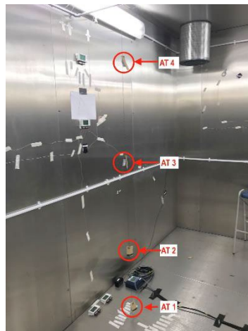
Air temperature sensors at different heights
