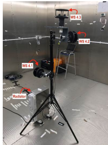
Air velocity sensors at different locations
